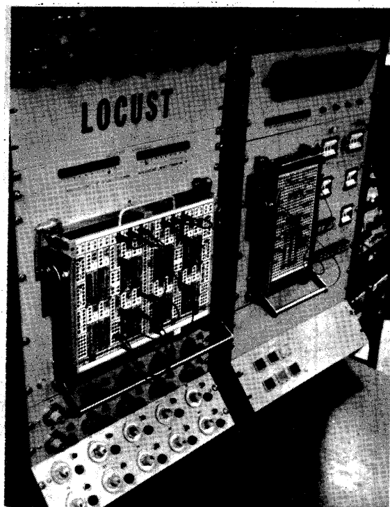
Figure 1—The LOCUST computer, built in the University of Arizona's Analog/hybrid Computer Laboratory. Linear and digital integrated circuits enhance computer performance and still reduce parts and assembly costs
